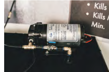
Custom built 12-volt diaphragm pump
