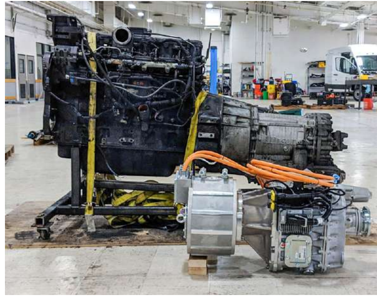
A diesel engine and transmission removed from a bus, and the electric motor and transmission that replaces it.
