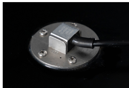
Hard cover to prevent physical damage or tampering
