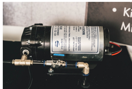
Custom-built 12 volt diaphragm pump
